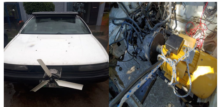
Figure 4 ; Mitsubishi Mirage with solar panel, electric motor and wind turbine to charge batteries
